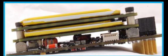
CubeSat Power board with integrated 20Whr battery
